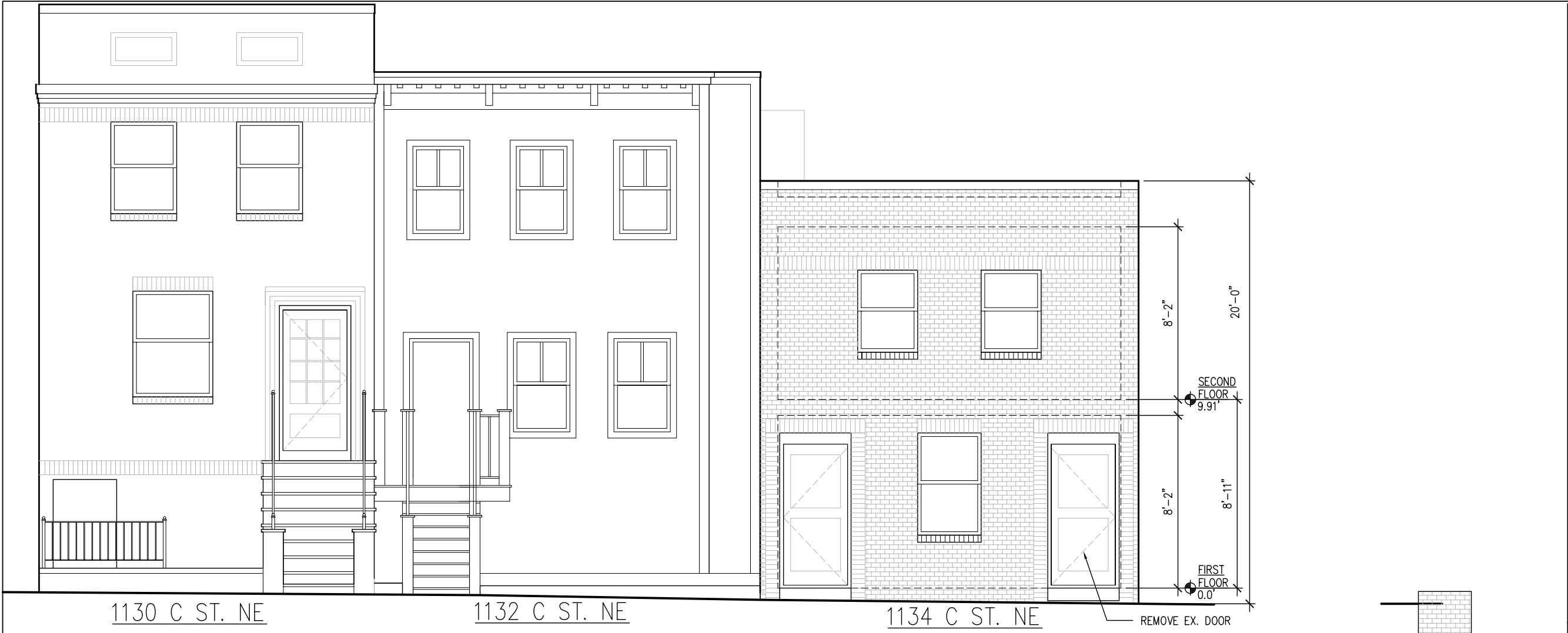
1 Existing / Removals Front (South) Elevation Scale: 3/16" = 1'-0"
