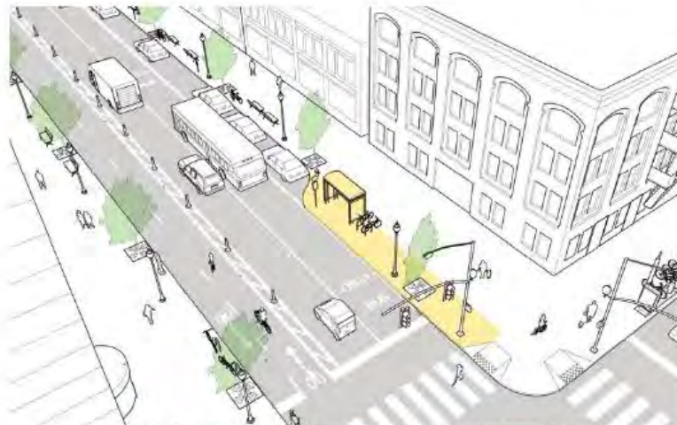
Figure 2: Examples of a bus bulb-out (source: NACTO.org)
