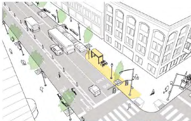
Figure 2: Examples of a bus bulb-out (source: NACTO.org)
