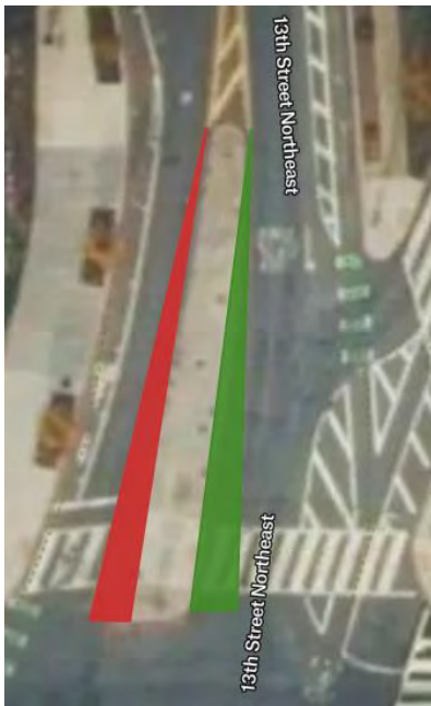
Figure 1: Recommended squaring of existing pedestrian island
